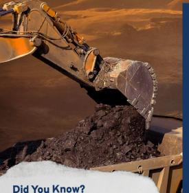
Excavators can only travel around 4km/hr and require rest breaks when 'walking' to avoid overheating the track gear.
