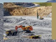
Open pit or surface mining involves excavating rock to reach the gold below the surface. The process follows a cycle of drilling, blasting, excavating, hauling, and rehabilitation to mine gold bearing rock.
